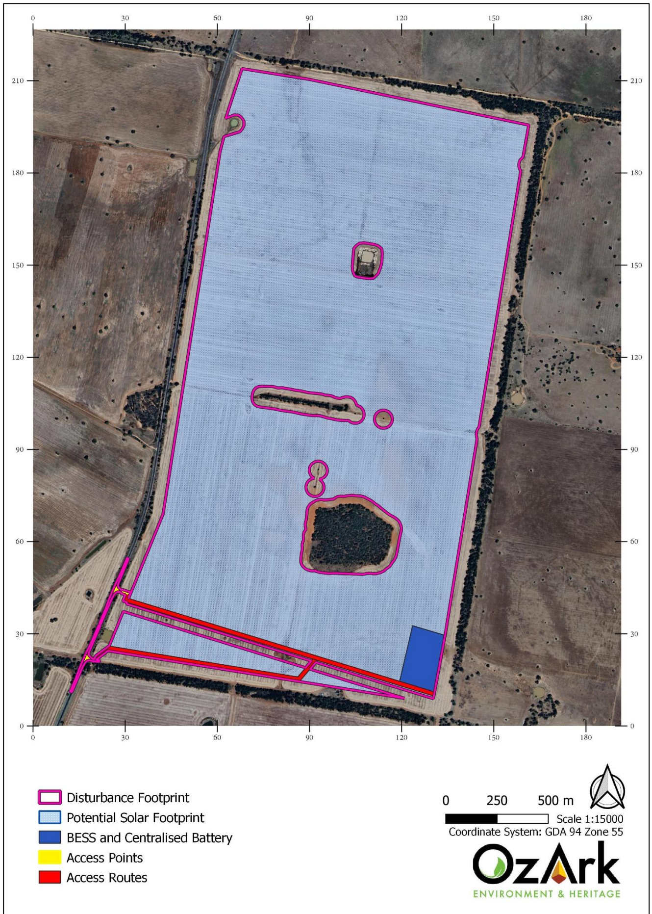
Figure 1-1. Proposed site layout for the Burroway Solar Power Station.
