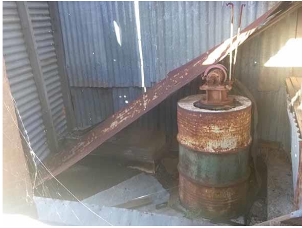
5. 44 Gallon drum with hand pump inside shearing shed
