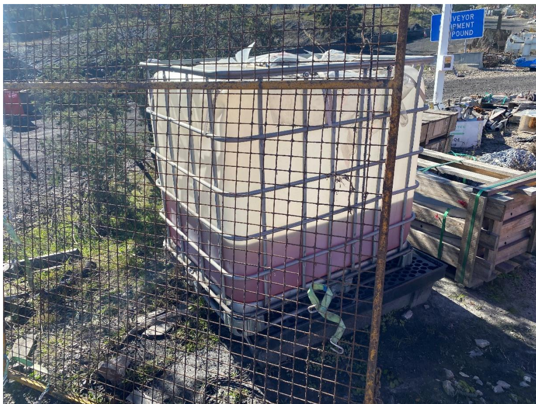
Photograph 12 – 1000L IBC containing hydrocarbons not stored as per AS1940
