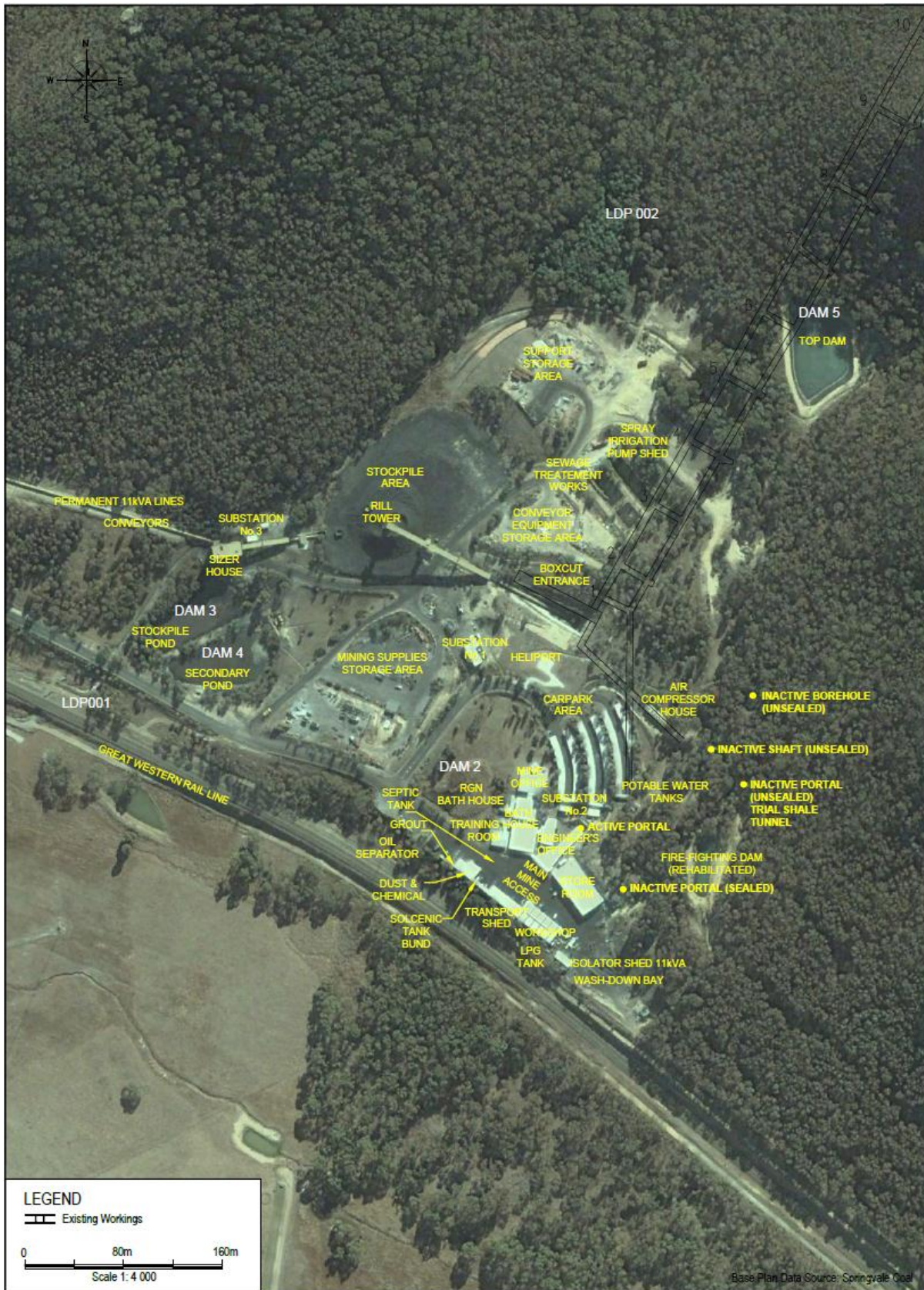
Figure 3: Springvale Mine Pit Top Layout
