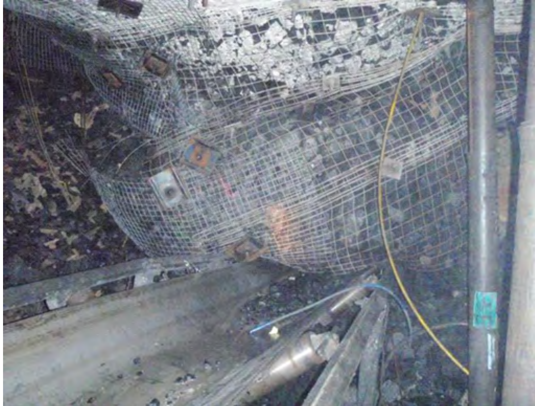
Photograph 8.1: Roof Fall on longwall belt at Springvale – approximately 6 m high and 20 m long
