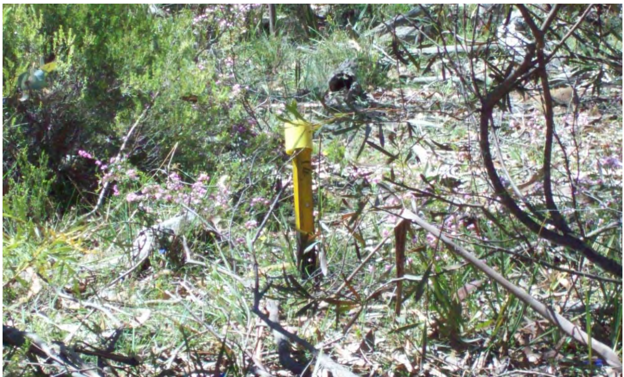
Plate 7: Subsidence Monitoring Peg
