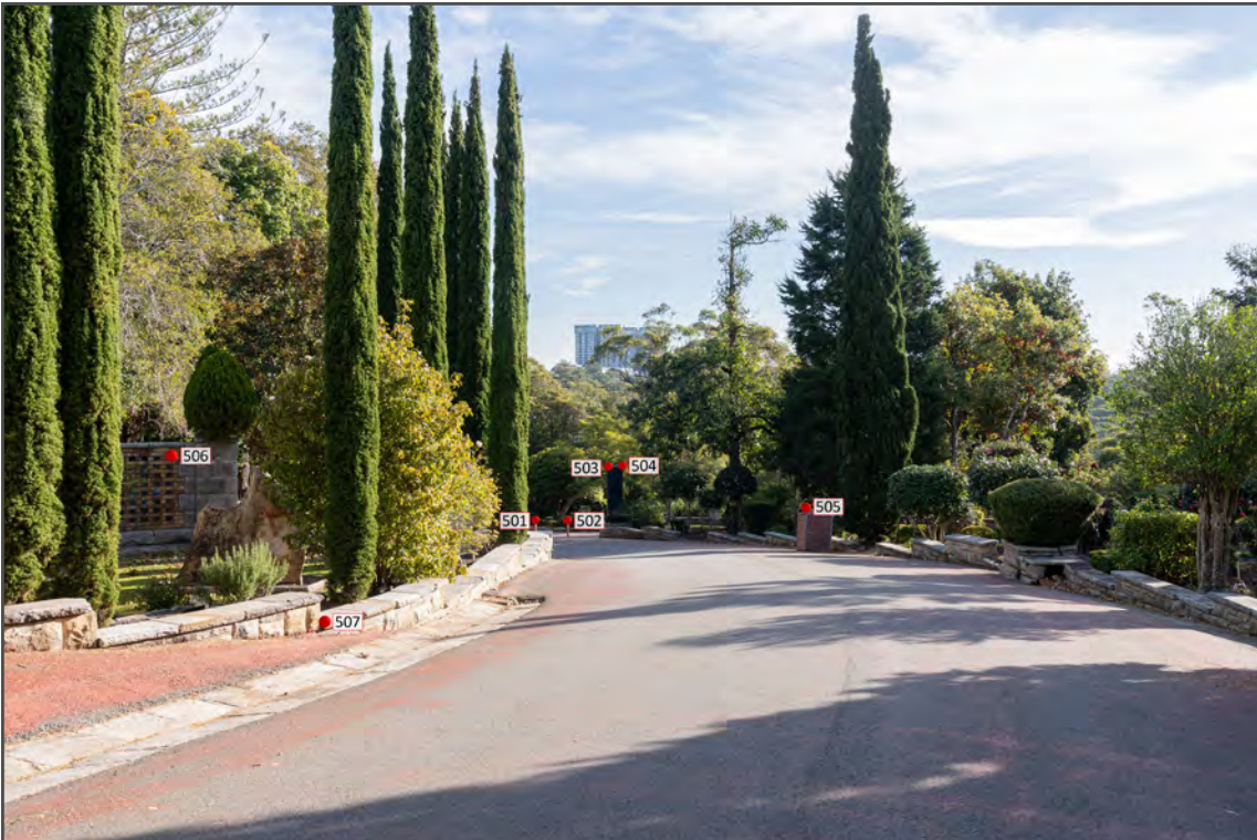
SURVEY POINTS USED FOR 3D CAMERA ALIGNMENT
