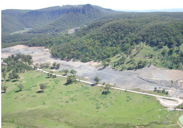
Plate 5.1: Shaped in-pit emplacement profiled to be compatible with adjacent undisturbed landform
