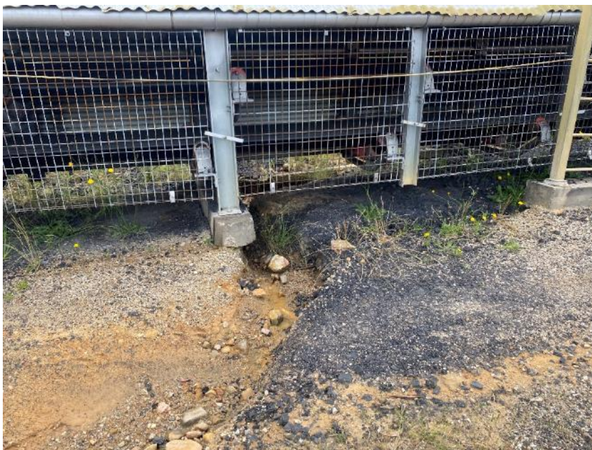
Photo 2: Coal to be removed from under some conveyors (refer IMP REC 15).
