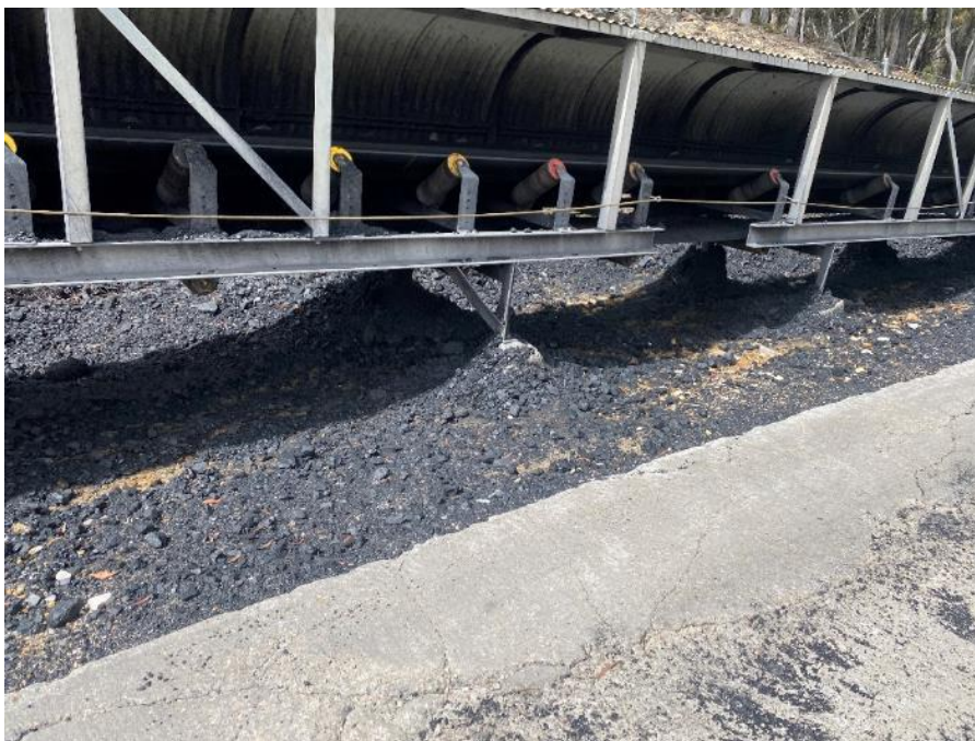
Photo 6: Removal of coal required under conveyors (refer IMP REC 15).
