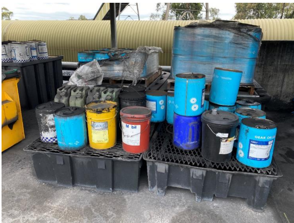
Photo 41: Hydrocarbons appropriately stored within bunded area at Western Coal Services Pit Top
