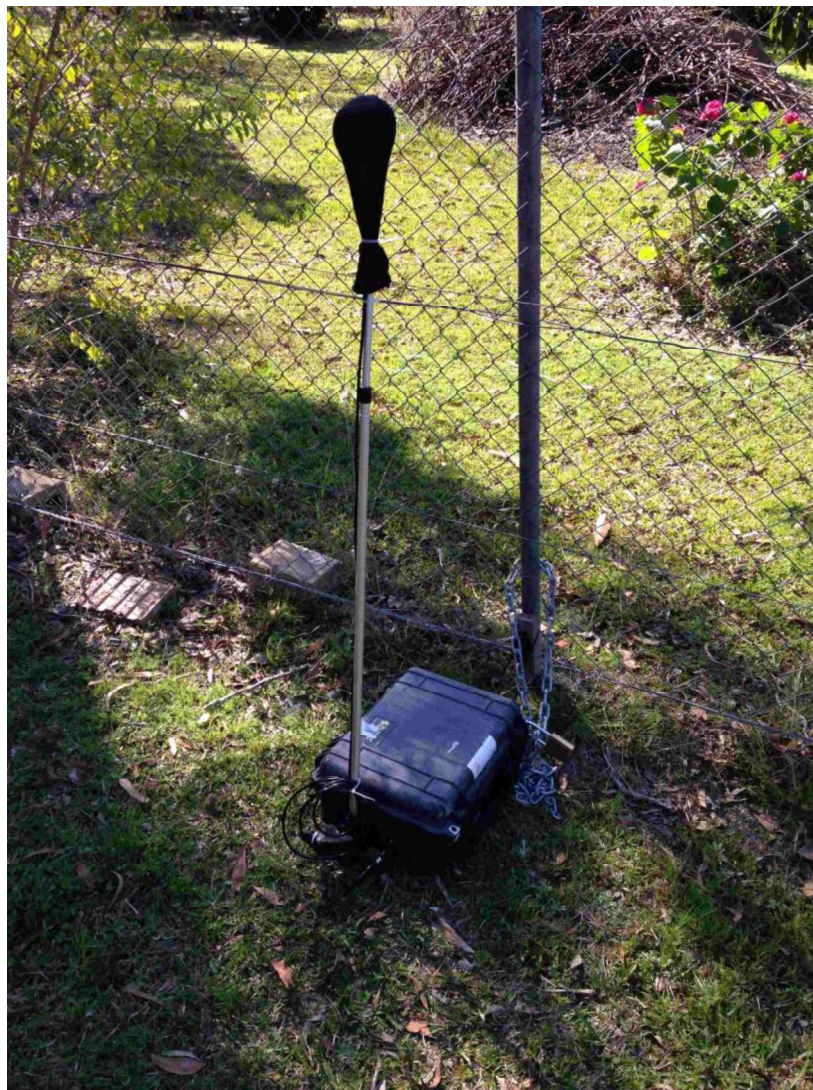
Figure 3 – Example unattended noise logger setup
