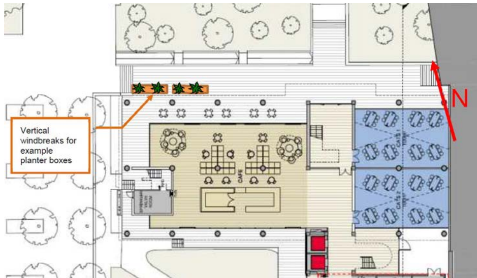
Figure 21 – Proposed window amelioration measures to Building J17.
