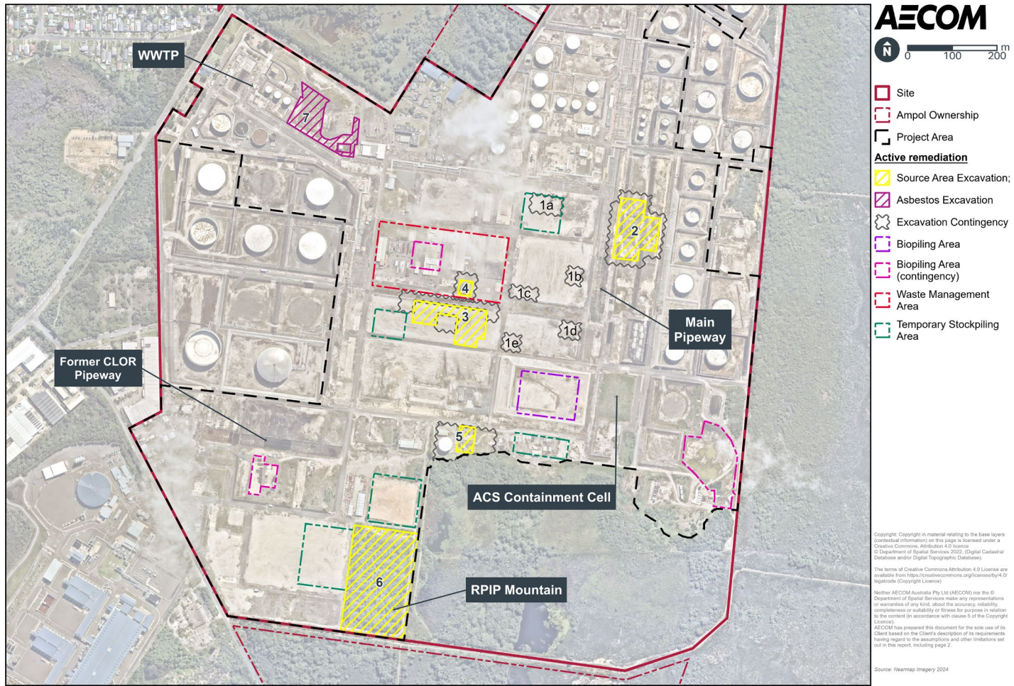
Figure 1-4 Targeted remediation activities (Stage 3)
