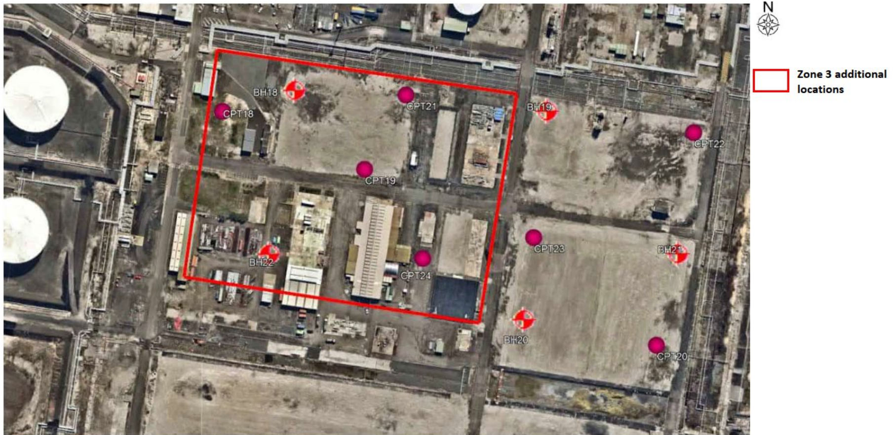
Figure 3-14 Geotechnical Investigation Plan – Zone 3 Additional Locations (WSP, 2023)
