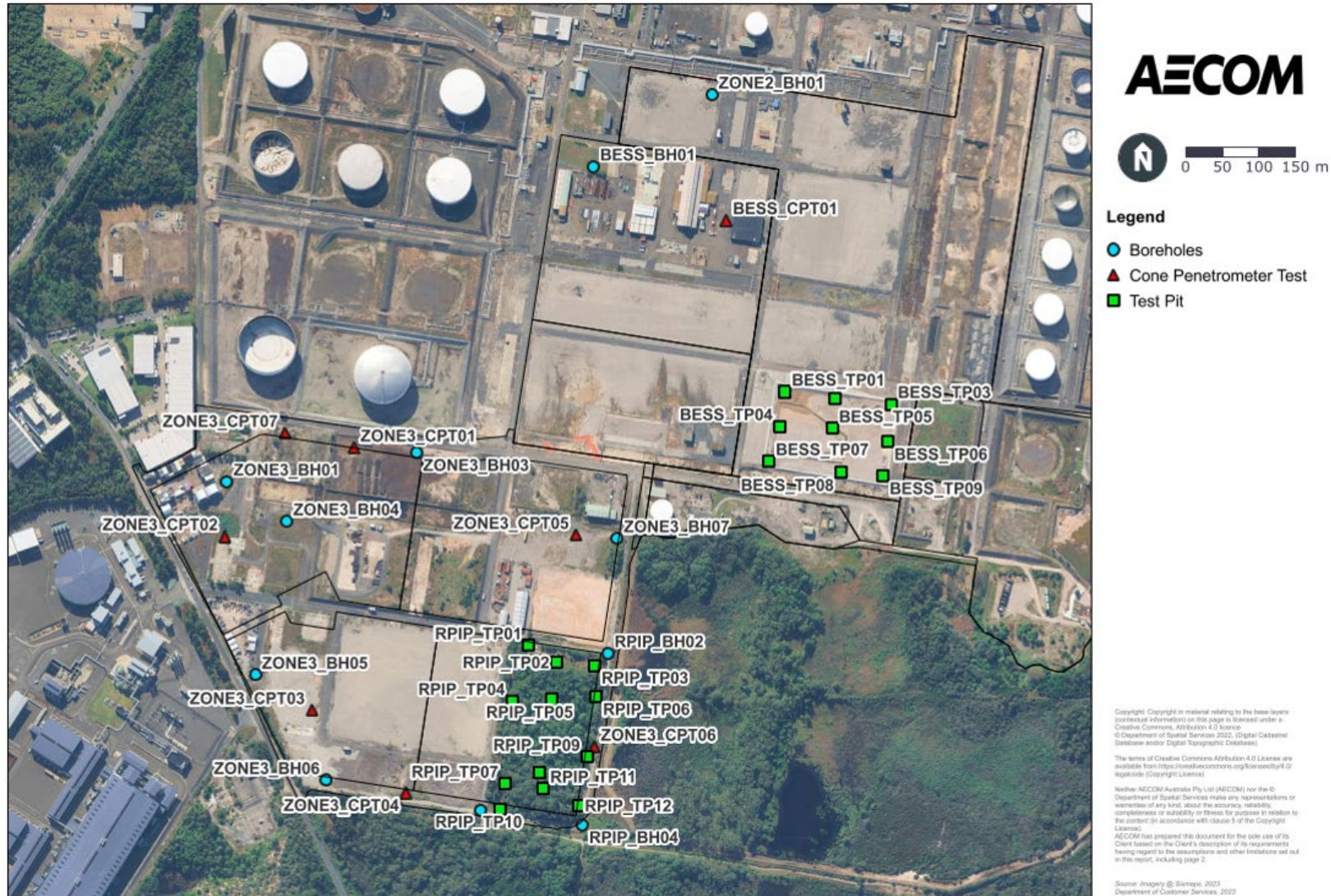
Figure 3-5 Geotechnical investigation layout (AECOM, 2025a and 2025b)
