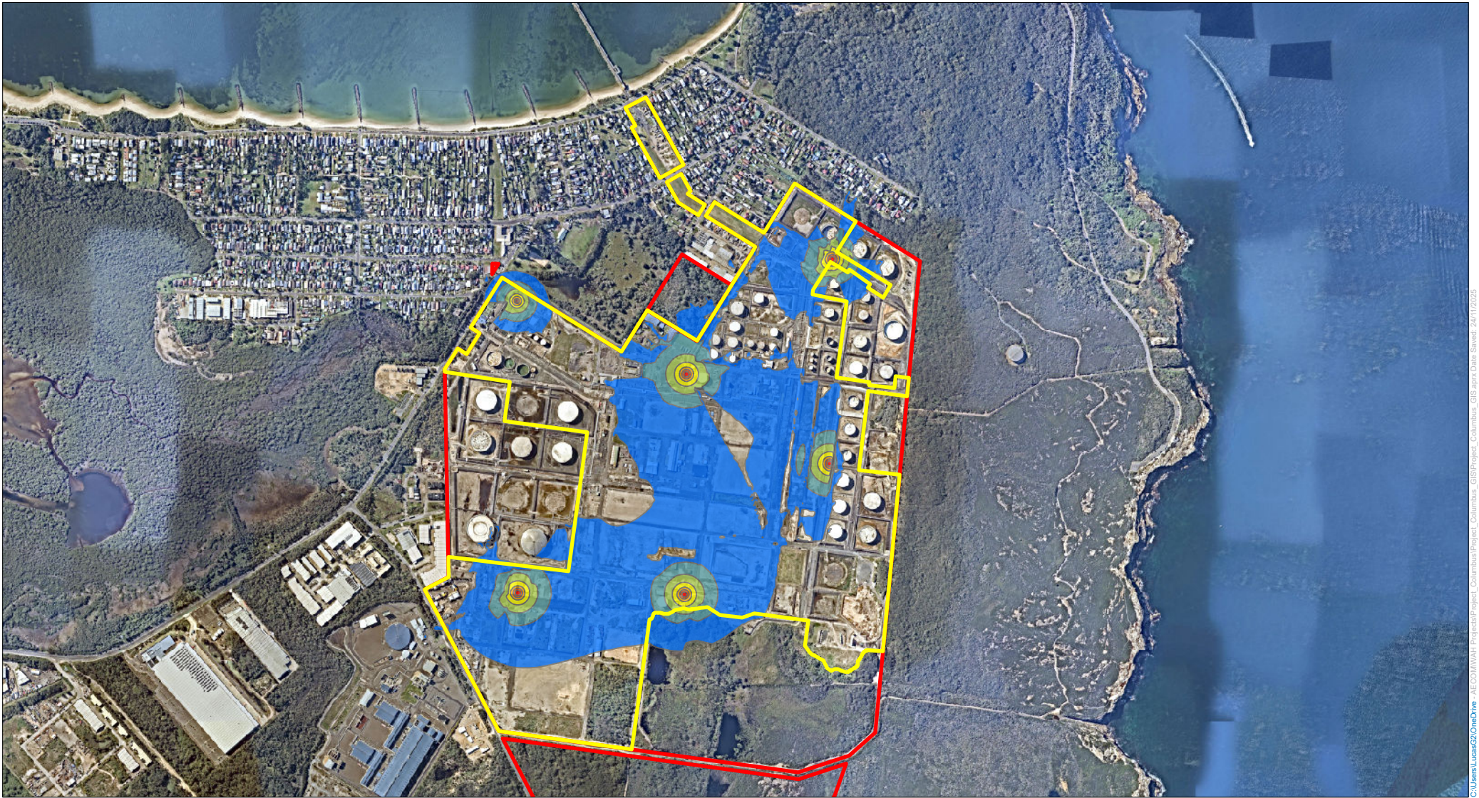
Construction Noise - Dewatering Pumps Noise contours are shown 1.5 meters above ground level
