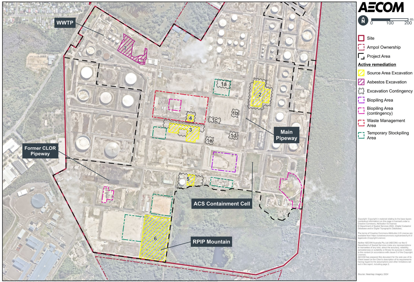
Figure 1-4 Targeted remediation activities (Stage 3)
