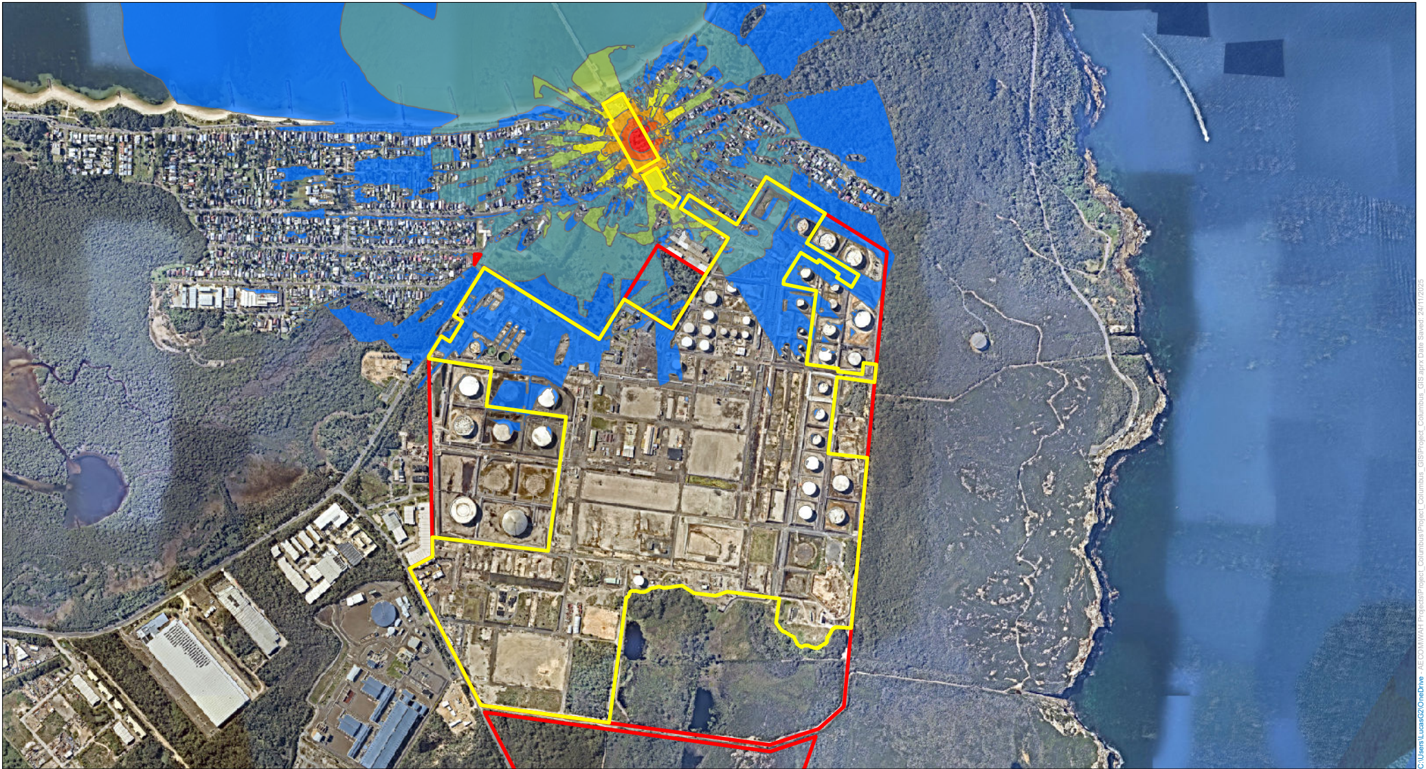
Construction Noise - Scenario 02 Noise contours are shown 1.5 meters above ground level
