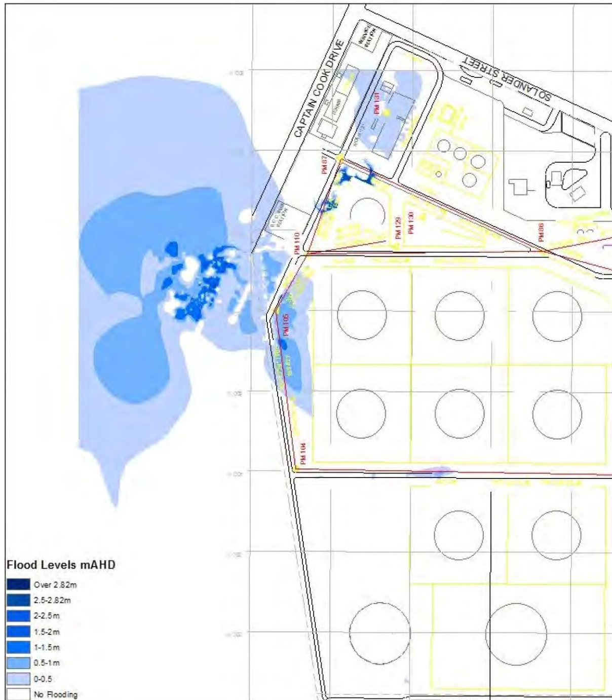
Figure 4-5 Extrapolated 1% AEP flood extents across the north-west corner of the Site (URS, 2013)
