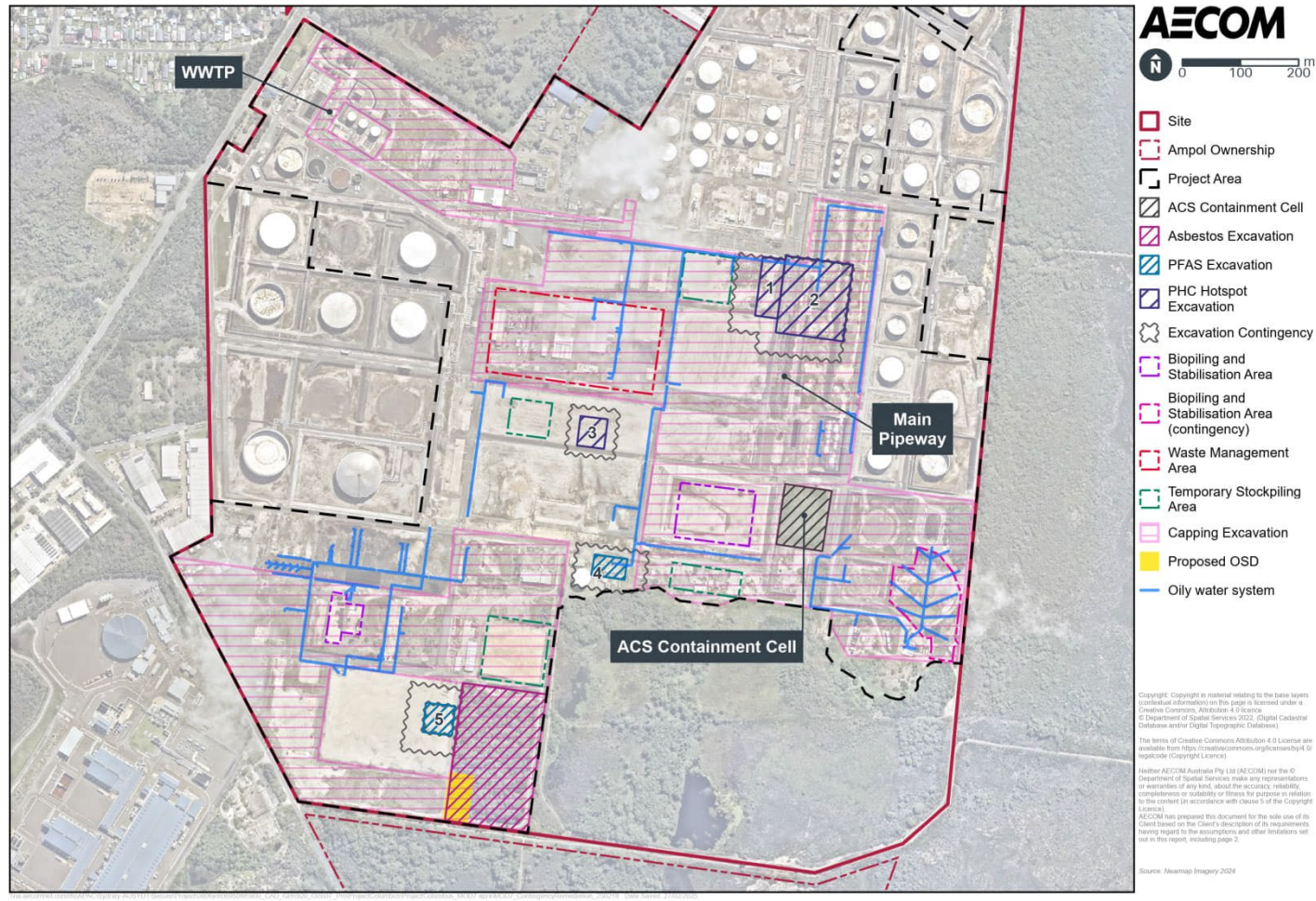
Figure 4-2 Excavation and excavated material management
