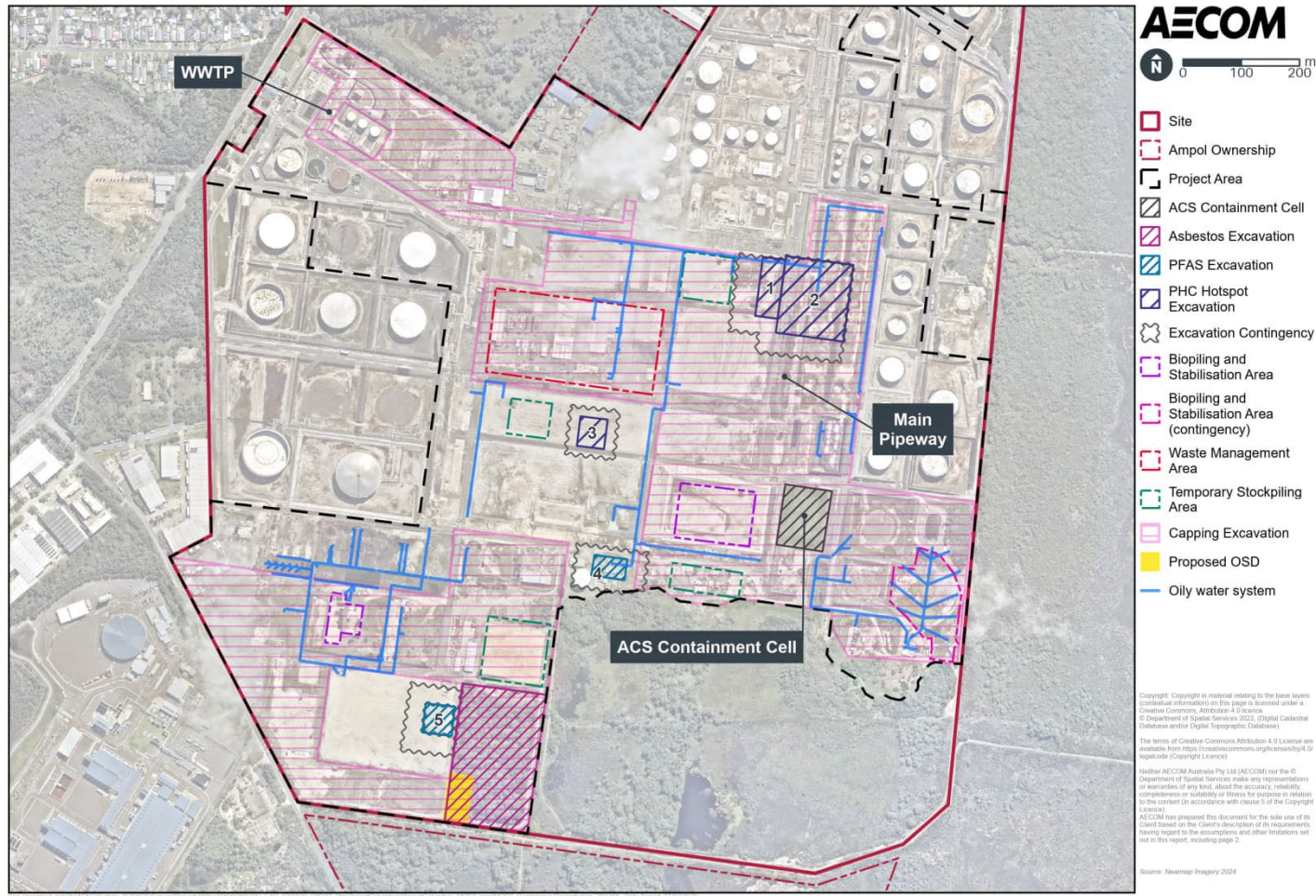
Figure C-18 Excavation and excavated material management
