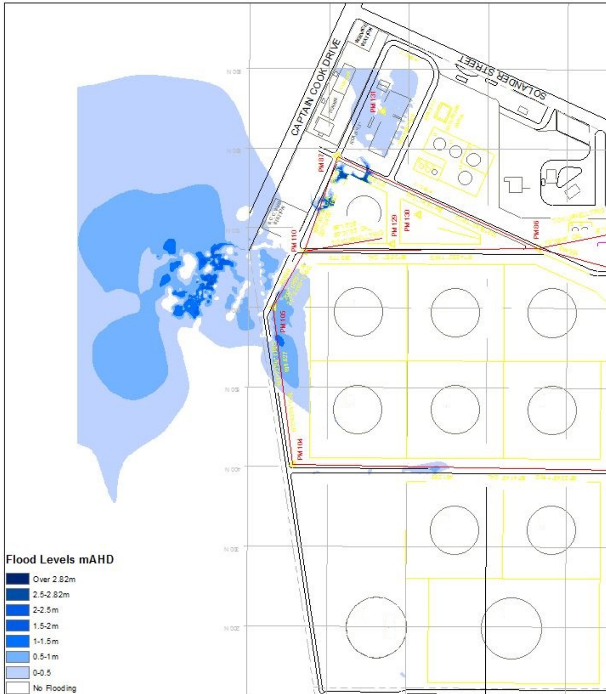
Figure 11-3 Flood Projection (2.82 m AHD) on the North West of the Site
