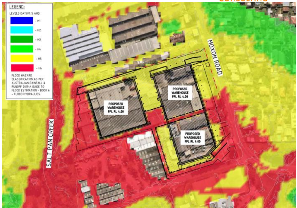
Figure 3.10: PMF Post-developed Hazard
