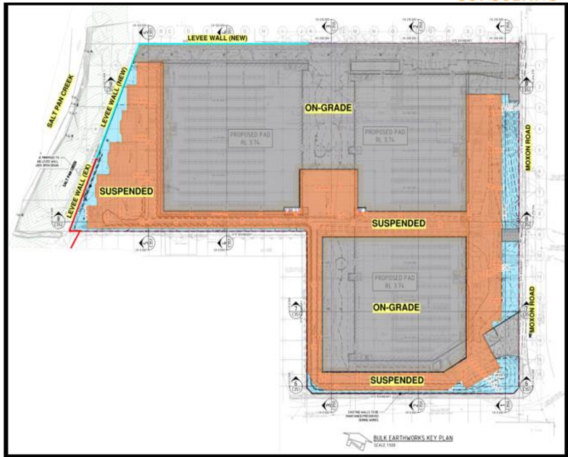
Figure 2.6. Finished Levels Plan – On-Grade and Suspended
