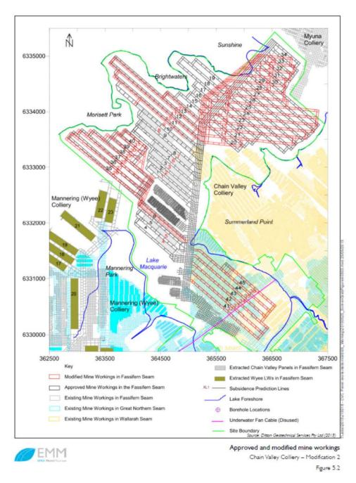
Figure 1: Plan showing proposed mining layout (from MOD2 EA)
