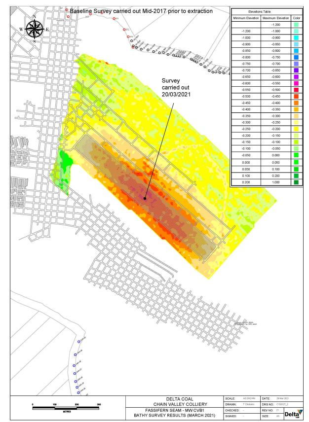
Figure 2 - Chain Valley Bay (MW-CVB1) Bathymetric Monitoring, March 2021
