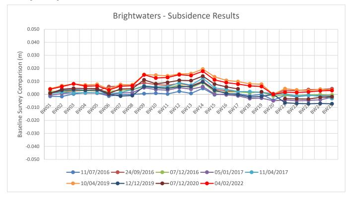
Figure 8 - Brightwaters Subsidence Results
