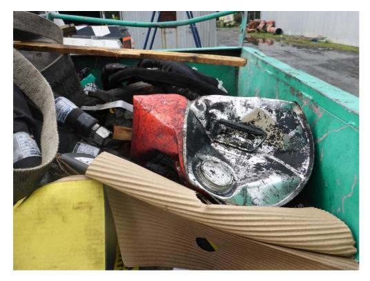
Photo 4 Hydraulic oil container should not be stored in general waste
