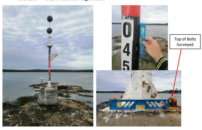
The levels for this survey are on Australian Height Datum, with the origin of levels being Permanent Mark 21207 with a recorded level of 6.831m.
