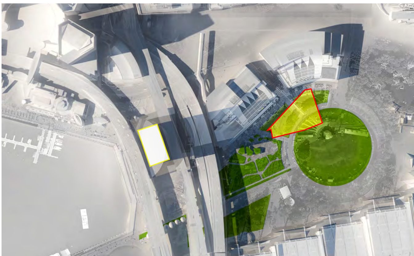
Shadow at 1 p.m on the Winter Solstice - 21st June. Approximately 12% additional shadow on green spaces as illustrated by the yellow hatch
