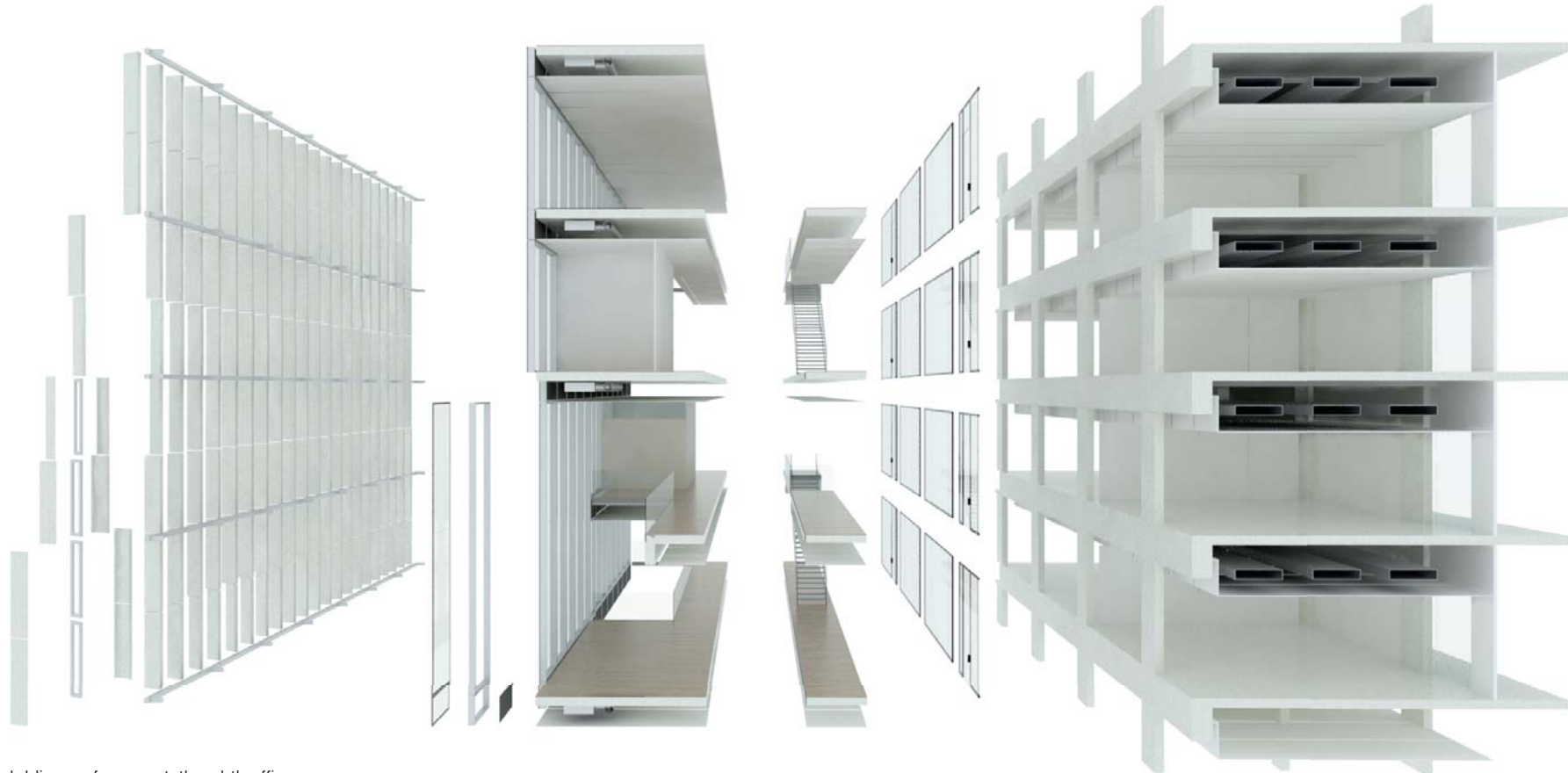
Figure 4.13 Exploded diagram of components through the office zone
