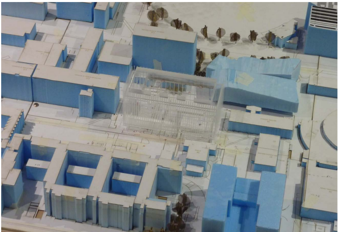
Figure 3 – Close up view from the north of the scale model of the UNSW campus and new MSE building in the wind tunnel.
