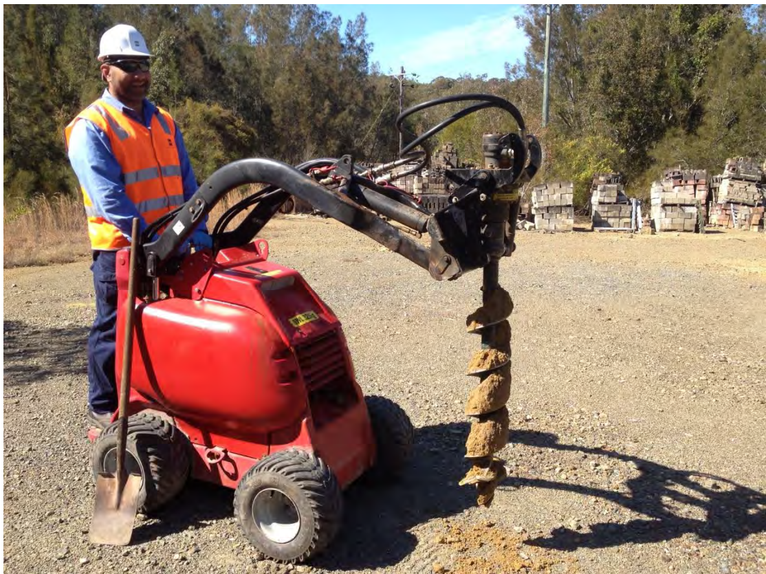
Photo 18: Dingo with auger used for soil sampling in areas of higher compaction.
