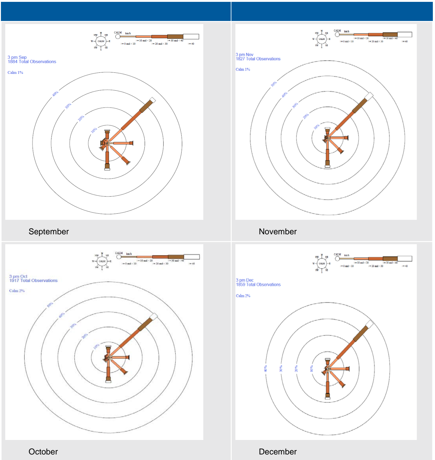
Figure 7-4 Average annual wind direction and speed for Coffs Harbour – 3 pm for September to December (BOM 2012)
