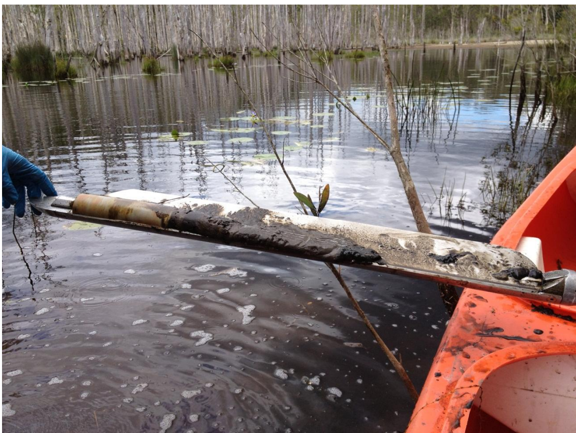
Photo 6: Sediment lithology at SE034 showing grey clay layer underlying organic matter and silty clay
