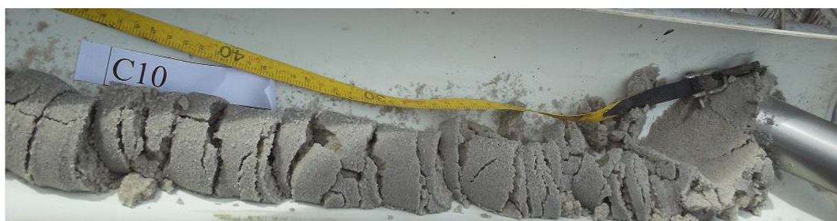
Photo 8. Unconsolidated soft light brown well sorted quartzose sand (<5% fine fraction and <0.2% TOC content) from C10 in fixed berth #1 (Dredge Area 3).
