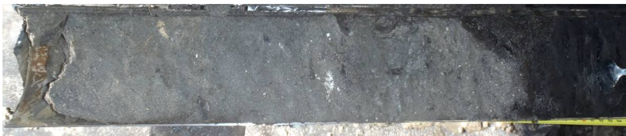
Photo 7. Silty sand overlying clay in VC5C (0.0 - 0.5m) from fixed berth #1 (Dredge Area 3).
