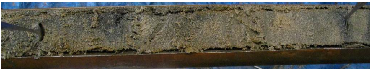
Photo 4. Silty sand in VC4B (0.5 -1.0 m) from the turning circle (Dredge Area 1).
