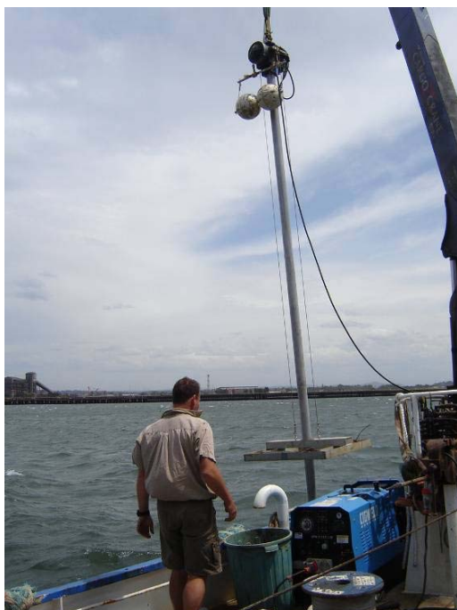
Photo 3. Use of the vibrocore frame.
