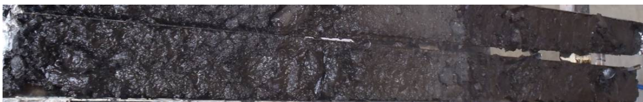
Photo 6. Fragmented peat/mud overlying clay in VC5E (0.0 - 1.65 m) from fixed berth #1 (Dredge Area 3).
