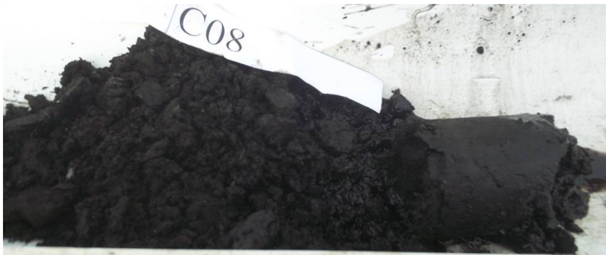
Photo 10. Consolidated very hard and stiff dark brown to black organic-rich flaky peat (dry in situ ) (47% fine fraction and 19% TOC content) from C8 in fixed berth #1 (Dredge Area 3).
