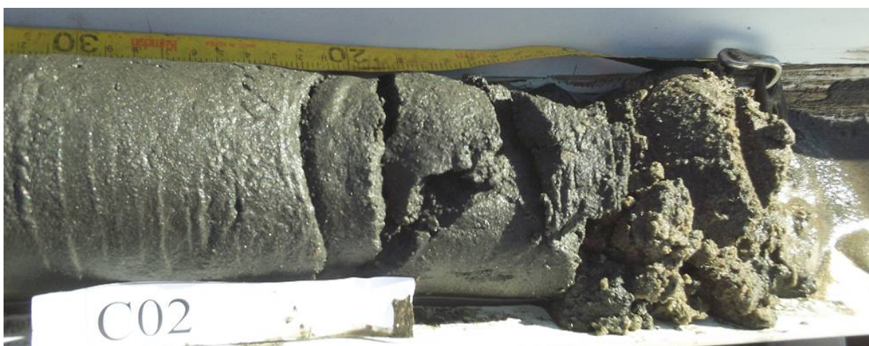
Photo 9. Unconsolidated soft dark olive-gray to brown muddy sand (20% fine fraction and 1.3% TOC content) from C2 in fixed berth #1 (Dredge Area 3).
