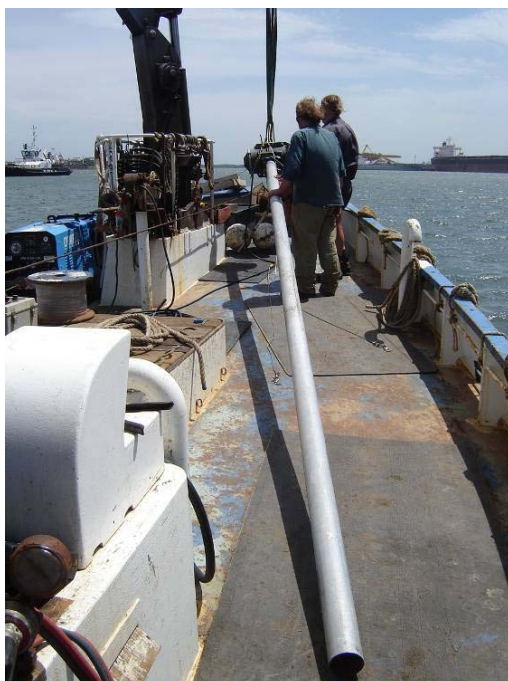
Photo 2. Vibrocoreing from the crane barge “Alkira”.
