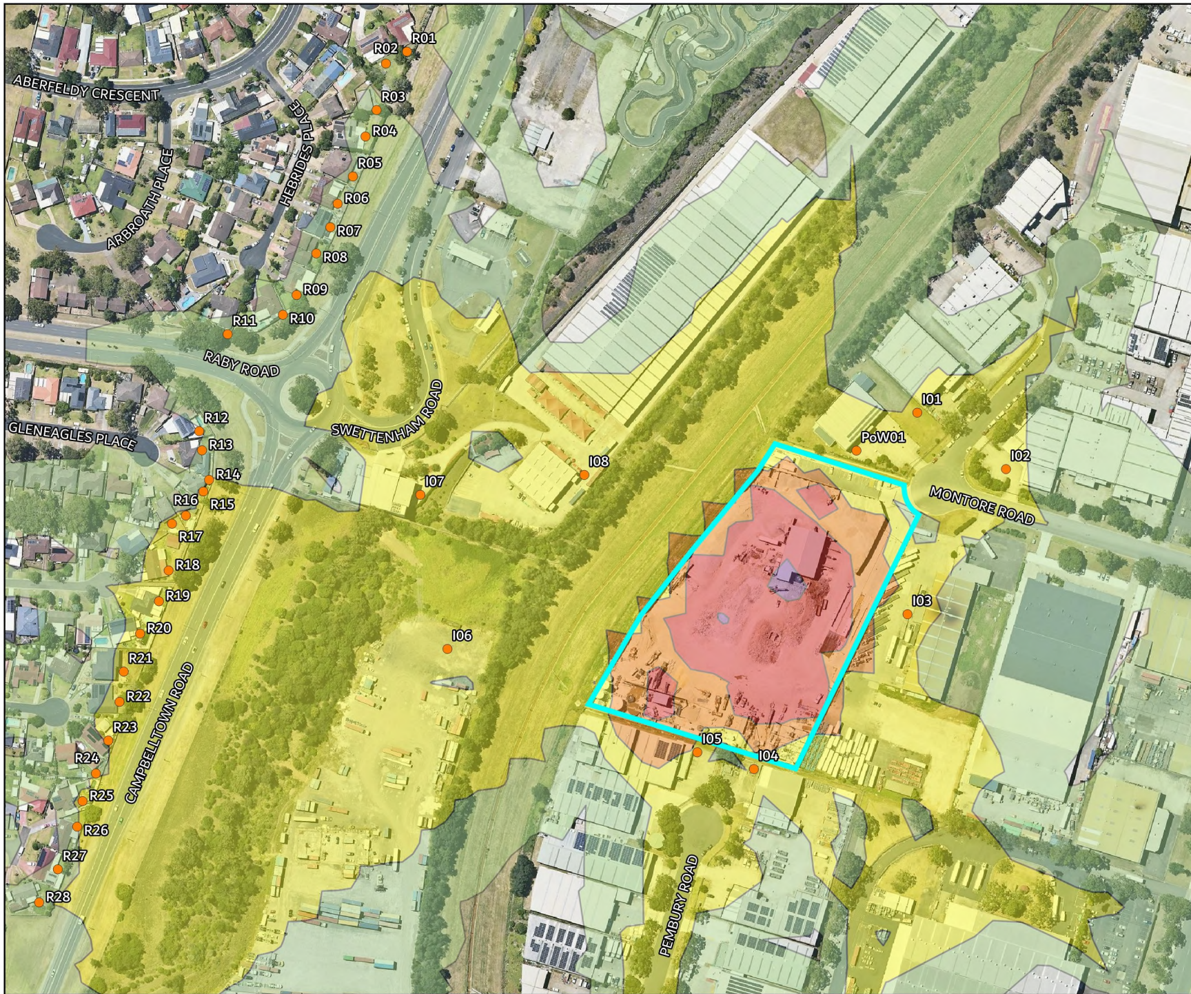
FIGURE 4 Noise Contours Day Operations MAC252458-01 Minto RRF 7 Montore Road, Minto, NSW Lot 52 DP 618900
