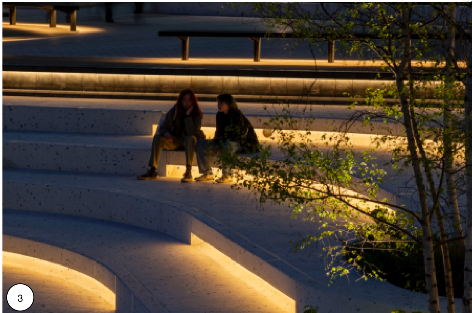
3 INTEGRATED LOW LEVEL LIGHTING FOR CONCRETE BLEACHERS/ SEATING ELEMENT FOR WAYFINDING/ DIRECTION AND TO MARK KEY GATHERING AREAS
