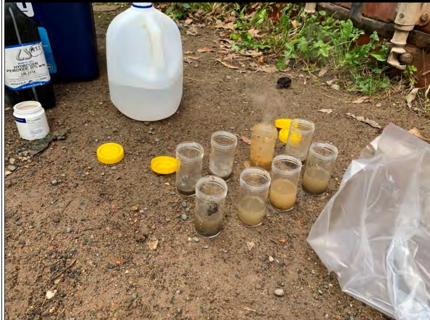
ONSITE ACID SULFATE SOIL FIELD SCREENING
