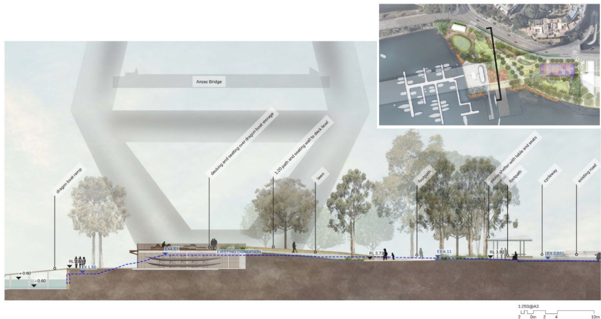
Figure 4.5 Section C (north-south section) through centre of Bank Street Park, showing the proposed reduction of ground level at the site of the proposed Dragon Boat Storage. (Source: Client provided)
