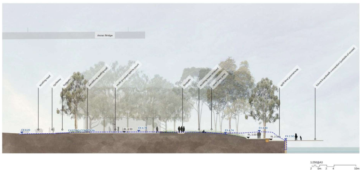
Figure 6.5 Section A through the eastern part of the site showing the final levels of the proposed park in relation to the present condition of the site (blue dashed line). (Source: Oculus, 2023)
