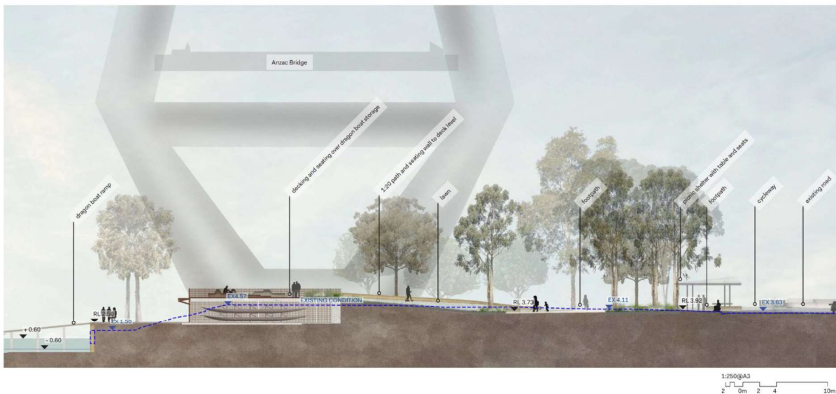
Figure 6.6 Section C through the centre of the site below the ANZAC Bridge showing the final levels of the proposed park in relation to the present condition of the site (blue dashed line). (Source: Oculus, 2023)
