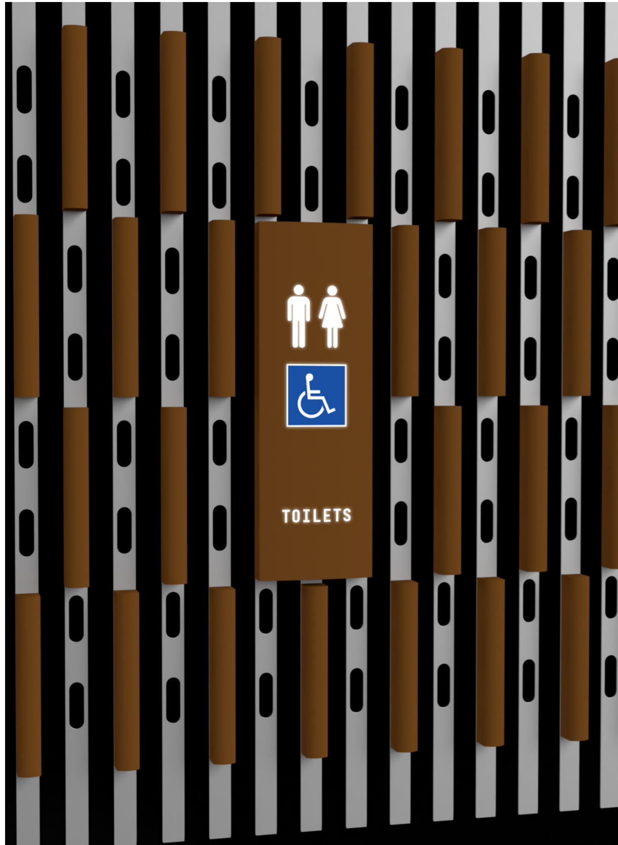
Custom tile to match the architectural facade tiling, with integrated lighting for clear visibility from distance day & night. Sign to be placed on amenity doors.
