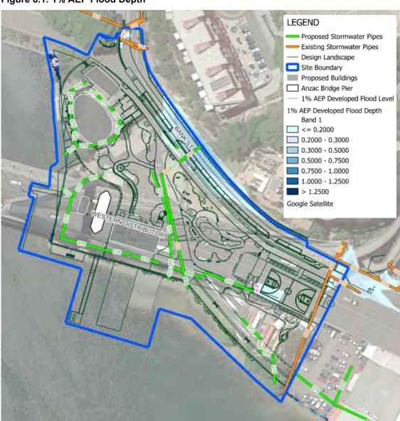
Figure 6.1: 1% AEP Flood Depth
