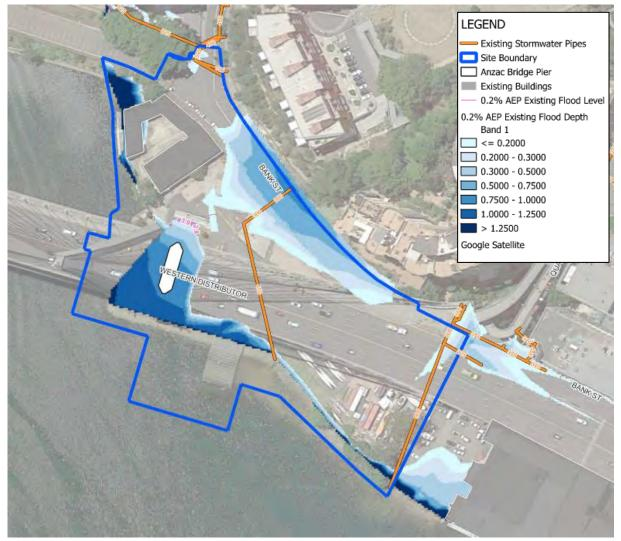
Figure 3-6: Existing 1% AEP Flood Depth with climate change
