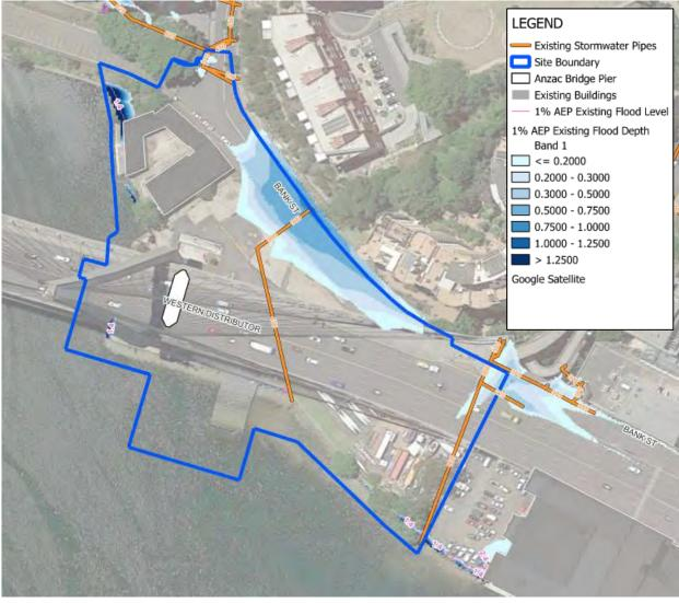
Figure 3-5: Existing 1% AEP Flood Depth
