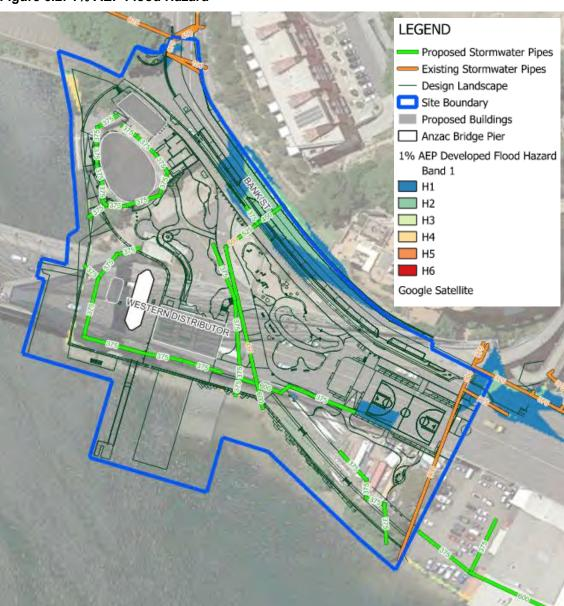
Figure 6.2: 1% AEP Flood Hazard
