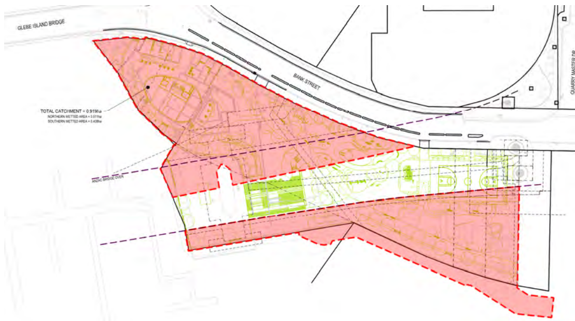
Figure 6 - Site Catchment (Wetted Area)
