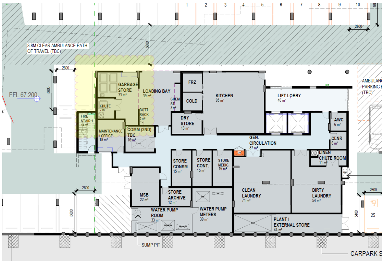
Figure 1 loading dock and internal waste (highlighted) area are concealed from the main road by a walled courtyard.
