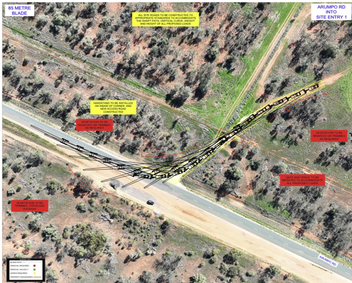
Figure 27 Additional OSOM Route Works – Access Point 1 / Arumpo Road Intersection
