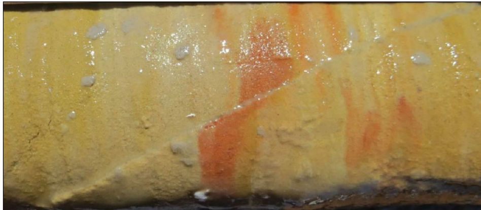
FIGURE 5.9. Defect in Cemented Sandstone Core from Borehole SAGT04 (Sonnekus 2015)
