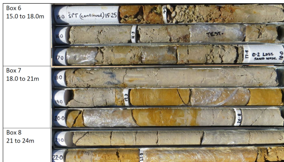
FIGURE 5.3. Typical Shepparton Formation Cemented Sand and Sandstone (Borehole SAGT01)
