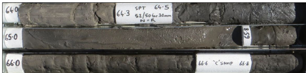
FIGURE 5.7. Ore Zone Core Photography Example from Borehole SAGT01 (Sonnekus 2015)
