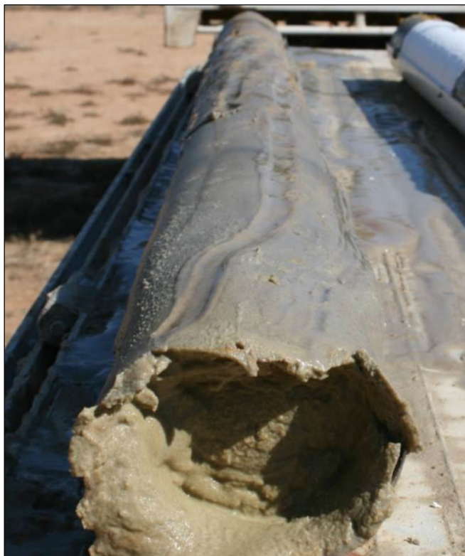
FIGURE 5.4. Core Slumping in the LPS1 as Observed in Borehole SAGT01 (Sonnekus 2015)
