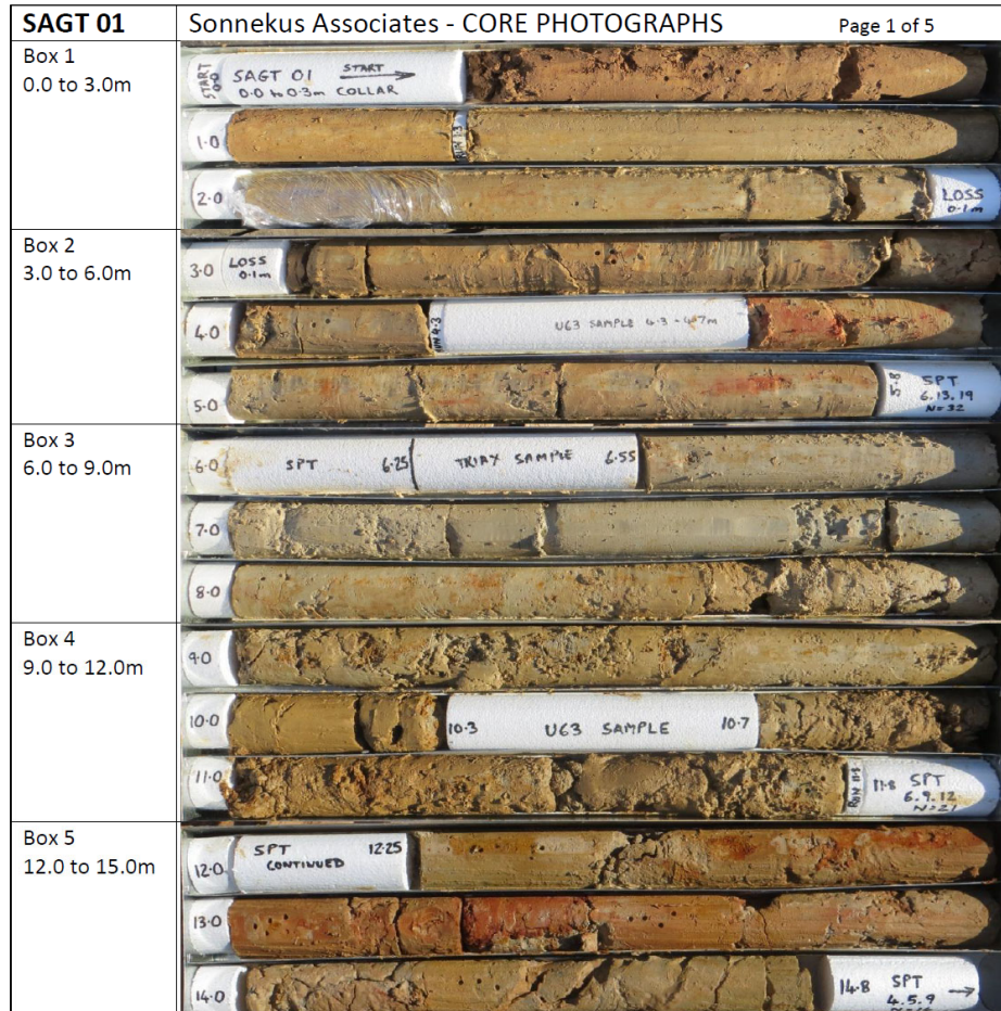
FIGURE 5.2. Typical Shepparton Formation Clays (Borehole SAGT01)
