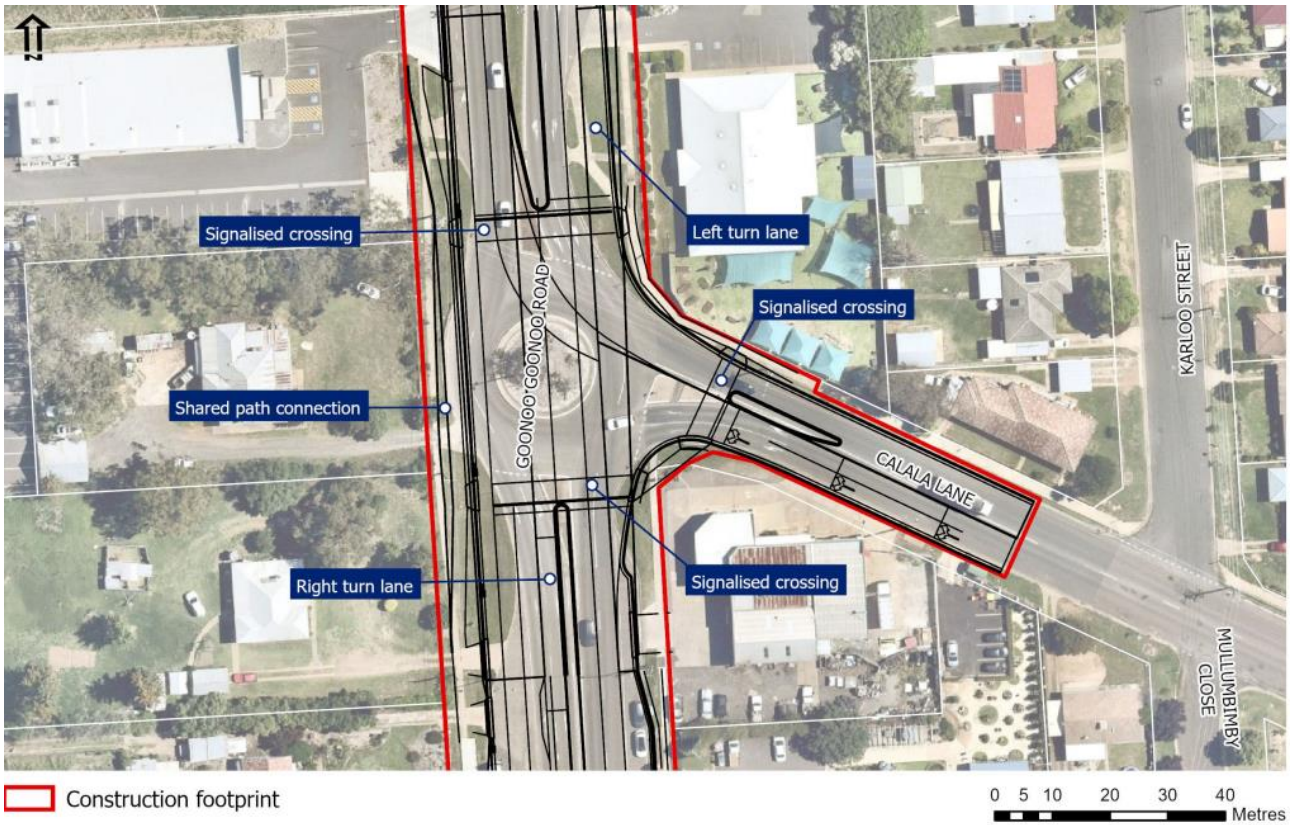
Figure 3:2 – Goonoo Goonoo Road/ Calala Lane intersection upgrade
