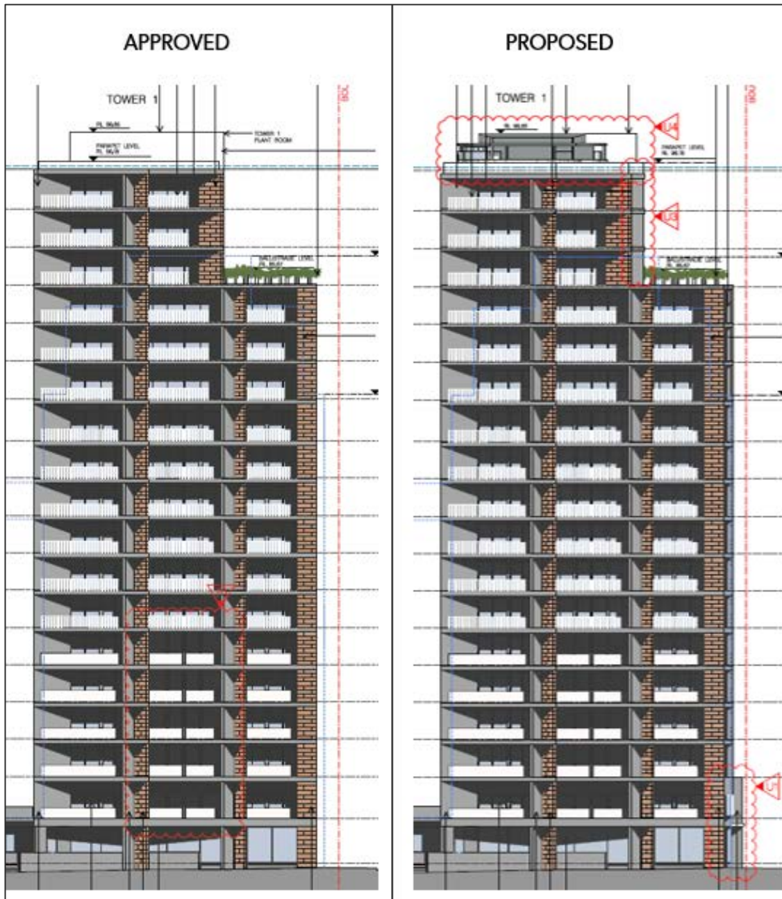
Figure 3 | North Elevation showing proposed roof terrace and balconies (Base source: Approved Plans MOD 7 and Applicant's Modification Report).
