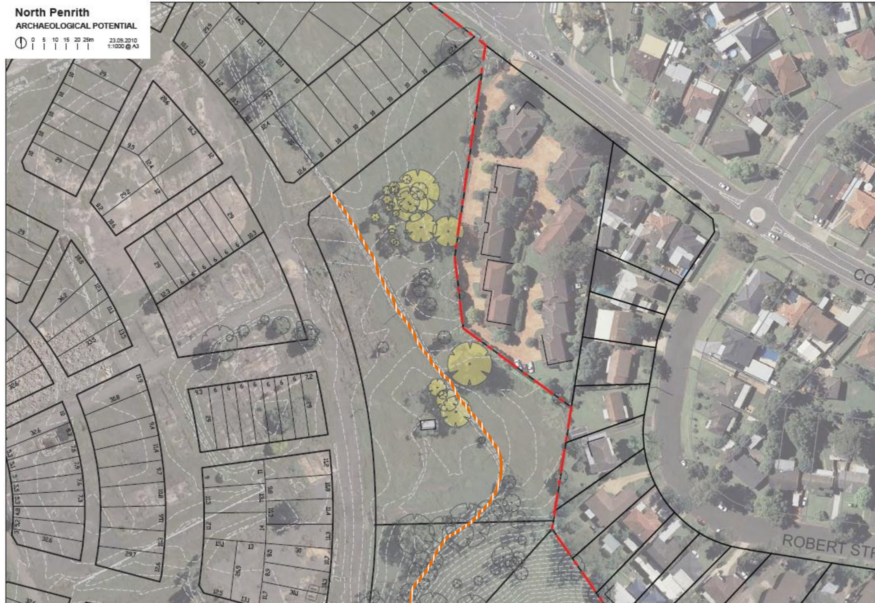
Figure 1: Section 88b areas within C3 lands. Orange, striped line represents approximate location ofswale assessed for this letter. Yellow indicates Section 88b areas
