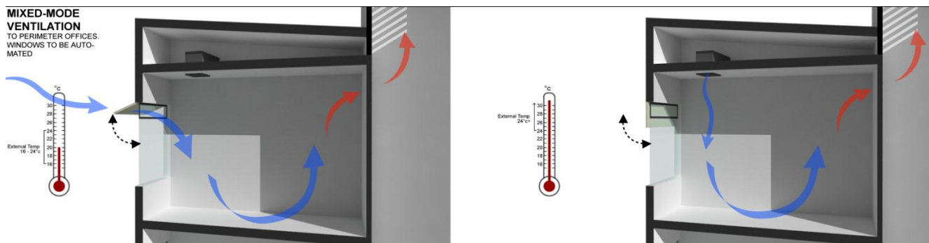
Fig: Schematic illustration of mixed mode ventilation.
