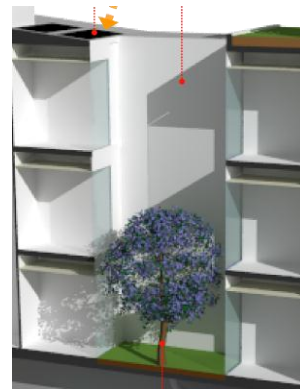
Fig 2: Voids and atriums can be incorporated to allow daylight harvesting to core spaces.
