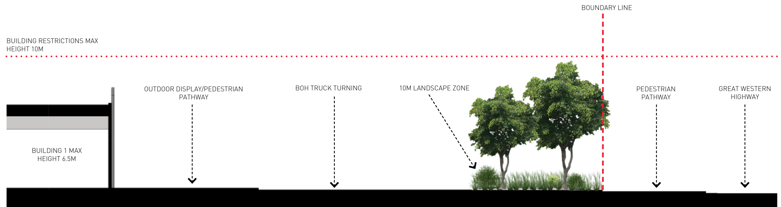
SECTION 6 - THROUGH BUILDING 1 TO GREAT WESTERN HIGHWAY
