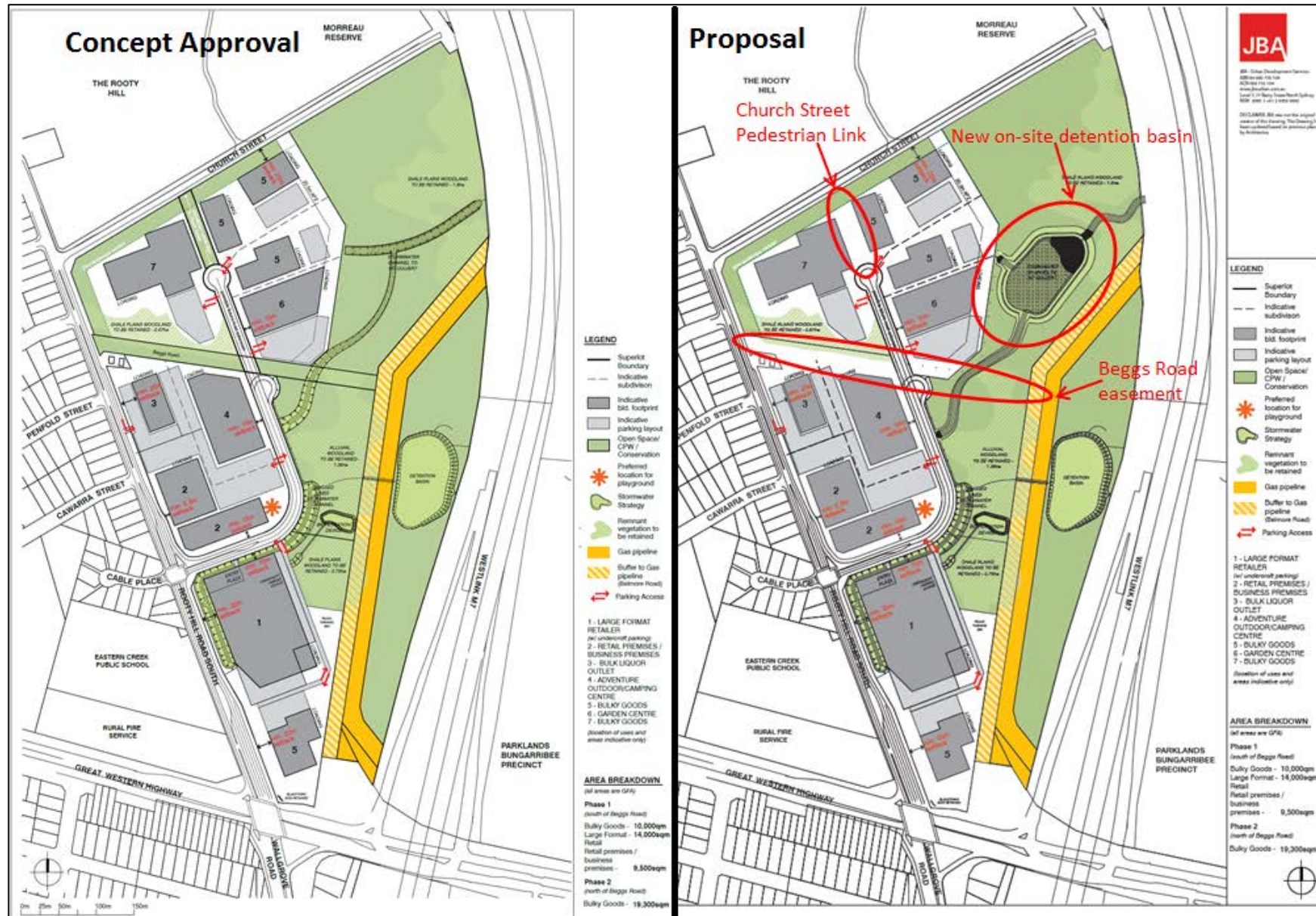
Figure 7: Comparison of approved (left) and proposed (right) layout of the business hub with proposed changes circled in red NSW Government Department of Planning & Environment
