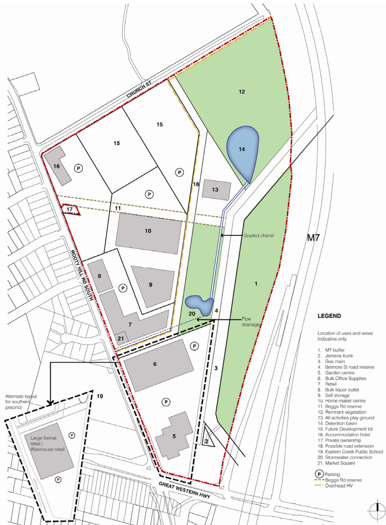
Figure 19 Indicative development footprint. A plan outline of building and activities possible under the future DA is illustrated.
