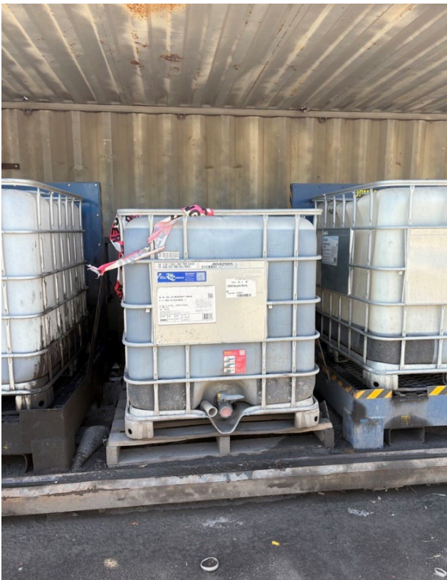
Plate 22: IBCs without bunding, however stored within shipping container (Inspection date 26/11/2025).
