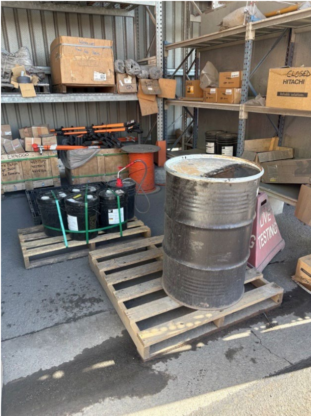
Plate 21: Workshop storage area with instances of unlabelled and un-bunded hydrocarbon and chemical containers (Inspection date 26/11/2025).
