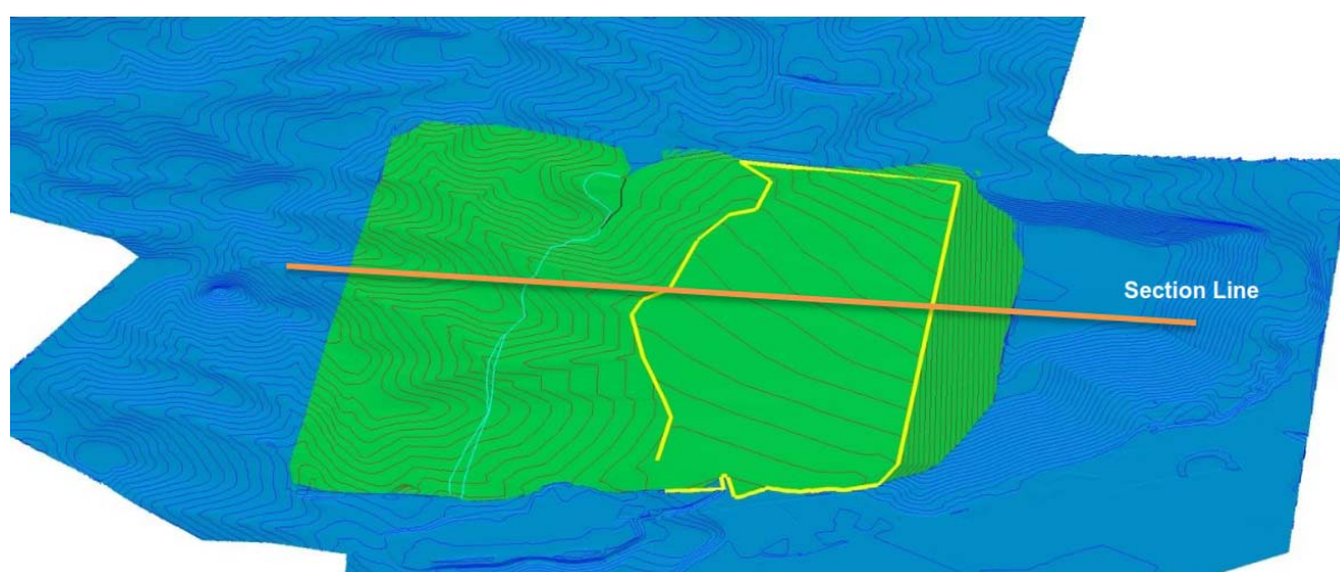
Figure 4 Back Fill to Original Surface (Option 2)
