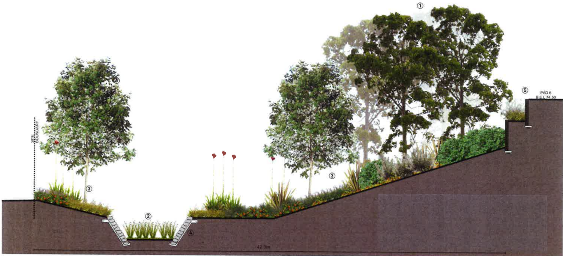
SECTION EE - Bioretention Basin 1:100
