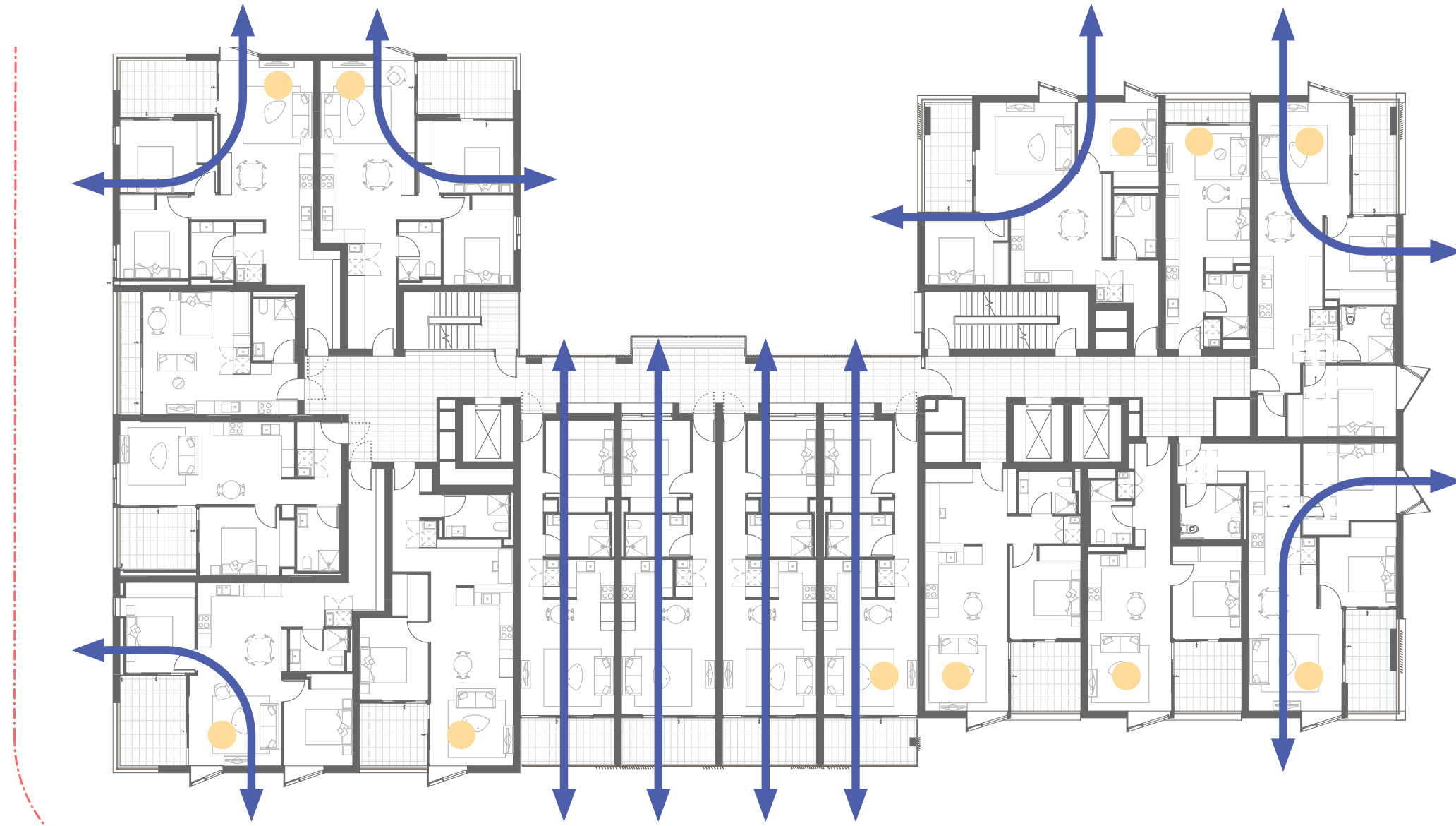
DAYLIGHT AND CROSS VENT
