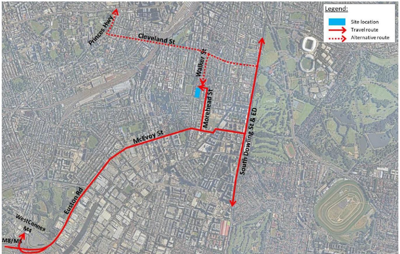
Figure 61 Anticipated construction vehicle routes
