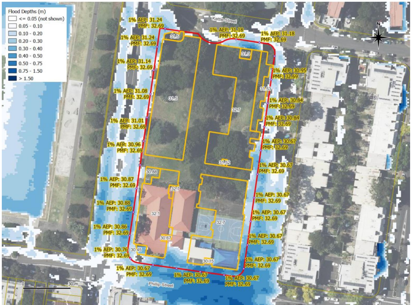
Figure 67 Post-development inundation during 1%AEP flood event
