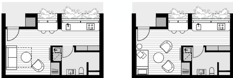
Figure 29 Building S2 – Compact Apartments – Layout Options
