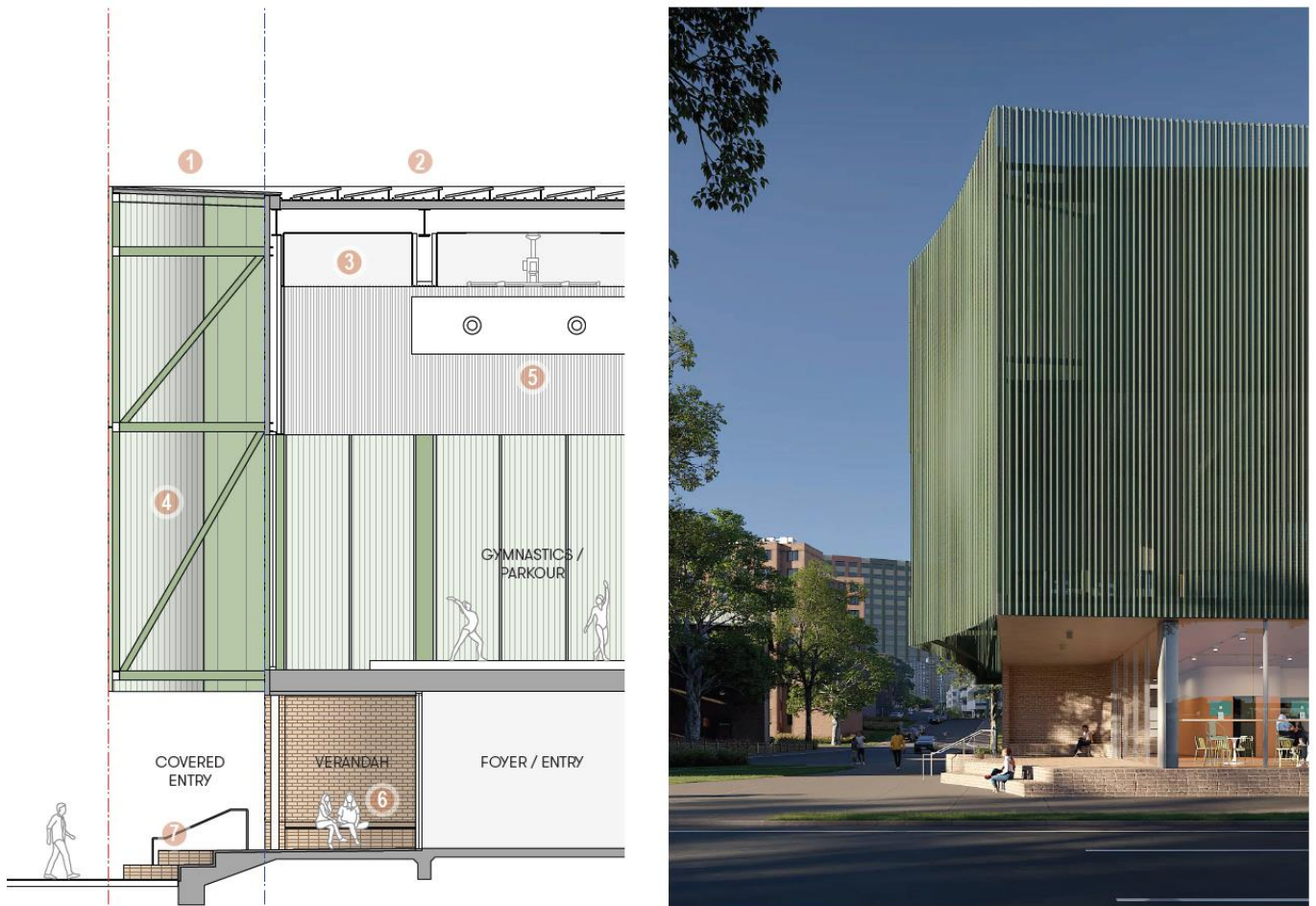
Figure 19 Building S1 – Northern Entry Façade and Materials
