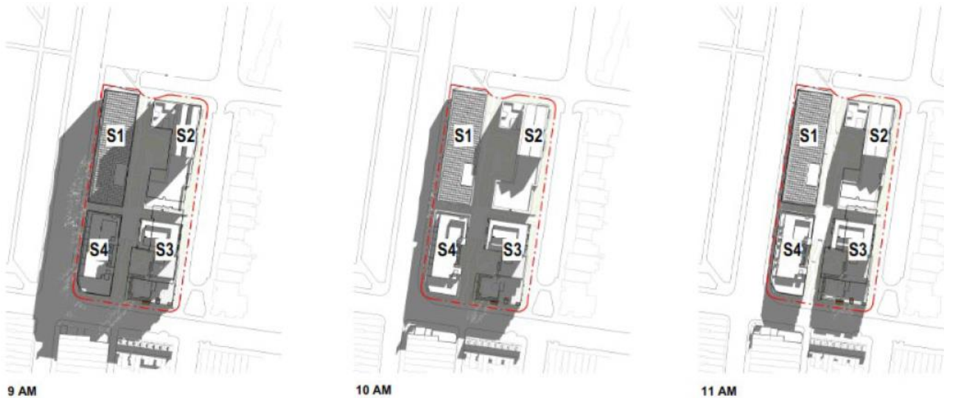
Figure 5 Mid-winter shadow diagrams at 9am, 10am, and 11am
